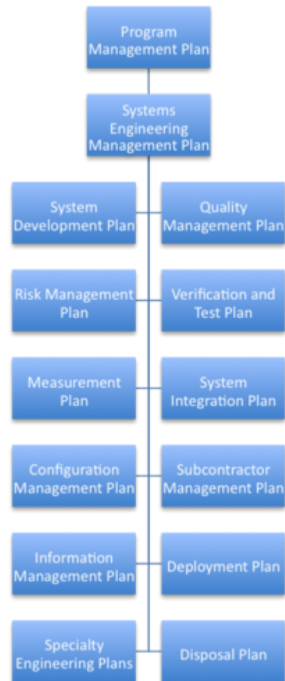
Figure 1. SEMP and Integrated Plans. (SEBoK Original)
