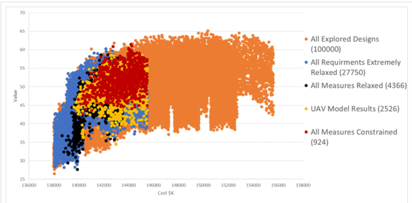
Figure 1. Effects of Requirements on the UAV's Feasible Tradespace (Parnell et al. 2019, used with permission)
